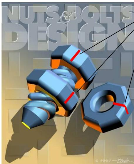
**Match marks are placed on bolts and nuts so that operator can easily detect if bolts have been loosen due to excessive vibrations. These are being placed on critical bolts after each bolt had received their correct torque.**
