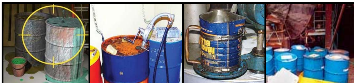
Bad and wrong practices on lubrication
